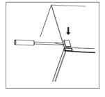
5. Move shaft sleeve and pin hole plug from left side to right side.
