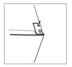
2. Remove the pin with a screw driver and flip the hinge bracket. Then refit the pin to hinge bracker.
