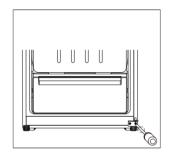
8. Unscrew and remove bottom hinge pin, turn bracket over, and replace it.
