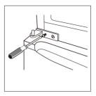
11. Place the upper door back on. Ensure the door is aligned horizontally vertically so that the seal are closed on all sides before finally tightening the top hinge. Then insert the top hinge and screw it to the top of the unit and then fix hinge cover by screw.
