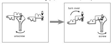
9. Refit the bracket fitting the bottom hinge pin. Replace both adjustable feet. Transfer the lower door to the proper position.
