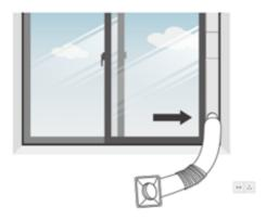
Step 5: Attach the hose connector to the exhaust air outlet of the unit.
